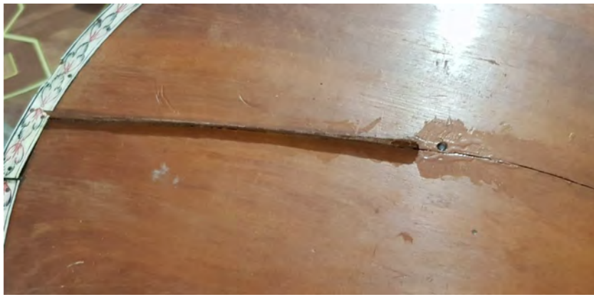
Fig. III.1.a The fixing the crack on the large resonator with a fragment of mahogany veneer.
